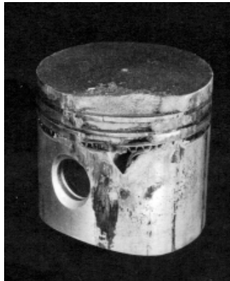
Detonation Damage (Hastings)
