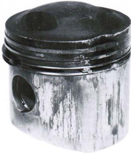
Mahle Fig 1-3 Detonation Damage
